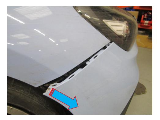
6. With the bumper separated from the vehicle, you will be able to see three plugs that need to be detached, one on the offside and two on the near side. At this point the bumper can be removed completely from the vehicle.
