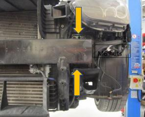
9. With the crash bar removed, place it front side down on the floor or work bench, looking at the crash bar with the lower support at the bottom you will see four predrilled holes to the right hand side. The four holes need to have the diameter increase to 12.5mm use the appropriate drill bit to achieve this.
