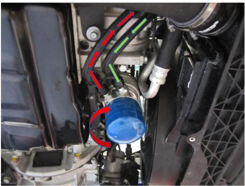
17. Run the hoses as shown in the pictures below, we would suggest you mark one of the hoses with a pen or pencil, so you know which the feed is and which is the return hose. The arrows in green show the feed direction and the red arrows show the return.
