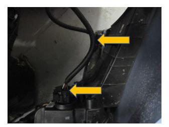
7. With the front bumper removed the first job is to unplug and remove the temperature sensor from the crash bar. To remove the sensor, use a trim removal tool or flat blade screwdriver to lever the sensor away from the crash bar.
