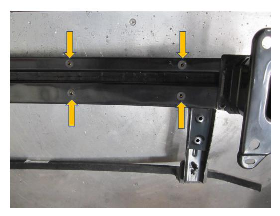
11. Offer the oil cooler and bracket to the crash bar and line up the holes in the bracket to the rubber riv nuts fitted into the crash bar from the previous step. Use the four M6x20mm cap head fasteners and M6 washers to secure the oil cooler into place using a 5mm Allen key to tighten them.
