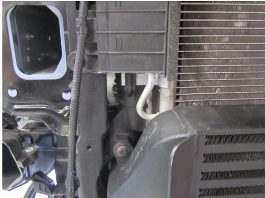
13. The next part to be trimmed is the plastic framework behind the area you just cut. As before measure and mark out the area to be cut then use a junior hacksaw to remove the marked area. These cut areas will allow better access for the oil lines to run to the oil cooler.
