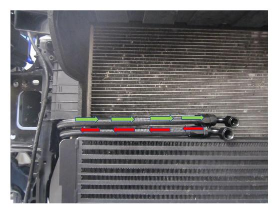
18. Offer up the crash bar with the fitted oil cooler to the front of the vehicle, attach the oil line to the oil cooler with the feed hose at the top and the return hose at the bottom of the cooler as shown below. Use a 22mm spanner to tighten the oil lines to the oil cooler, make sure they are tightened firm and fully. Once the oil lines are secure mount the crash bar back in place by following step 8 in reverse.
