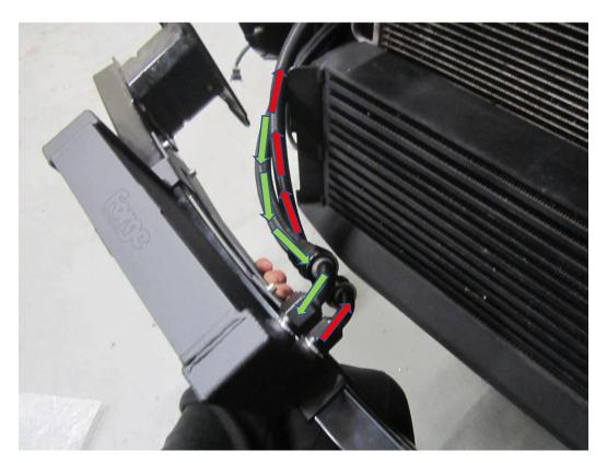
19. Use the supplied cable tie to secure the two oil cooler lines to the high-pressure hose below them. This is to avoid the oil lines chafing against the compressor.
